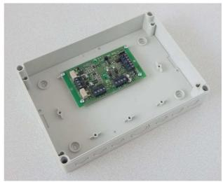
MHY 926 is an addressable multi-fold input/output element that connects to analogue addressable control panels of FDFAS LITES MHU 115, MHU 116 and MHU 117.
