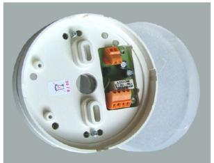
The base is supplied with 24 V. AC or DC voltage. The voltage is rectified and stabilized to supply the detector. If the detector is activated to the alarm state, the relay closes in the socket. The independent changeover contact of the relay can be used to control eg a fire shutter. The reset is performed by disconnecting the power supply.
