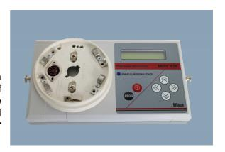
The preparation is intended for change of an address, parameters and checking of interactive fire detectors, interactive action units, addressable unit, technological units and linear smoke detector of analogue fire detection and alarm systems LITES. Allows checking of quiescent current of all detectors and motoric adjustment of optics in linear smoke detector MHG 664. Can also be used for checking of older types of addressable and nonadressable detectors.
