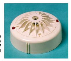
The MHG 331 Combined Temperature Detector is designed for places where in case of fire a temperature rise or a sudden temperature increase can be anticipated. This detector responds to a reached temperature rate or to temperature changes before and during a fire.
