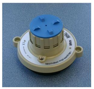
lonization smoke detector MHG 186 is intended for use in areas protected against atmospheric conditions and wherever it suits its coverage and climatic resistance and where there are no sudden changes in temperature leading to sweating and icing. Ionization smoke detector MHG 186 complies with the ČSN EN 54-7.
