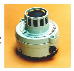
A robustly built detector operating on the principle of infra-red light scattering on smoke particles is primarily intended for explosion and fire hazardous areas with combustible gas, fumes, dust and explosives as well. It is also well-suited for common environments where higher mechanical and weather resistance is required.
